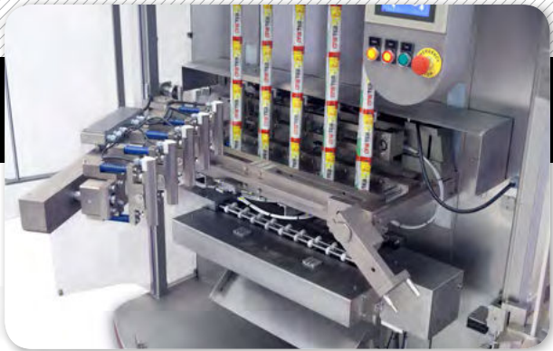
2. Twinpack sealing system.
