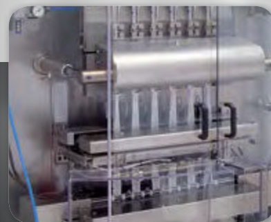
3. Independent sealing jaws.
