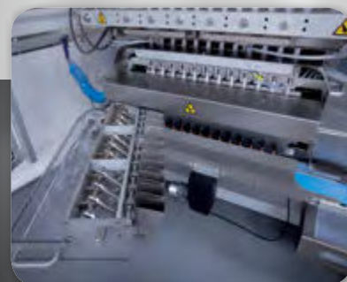
3. Independent rejection system.
